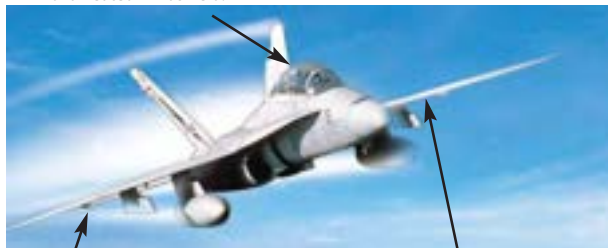
Flexible Thermal-Ribbons sense wing surface temperatures for wing surface de-icing.
